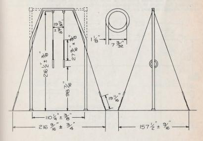
Article 3. Material for rings shall be unfinished hardwood and material for adjusting straps shall be webbing or leather. Hanging cables shall be a minimum of 4" diameter steel with a minimum tensile strength of 1323 pounds.
