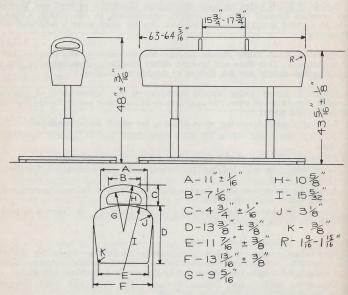
Article 2. The distance between the pommels shall be adjustable to any position from 15%" to 17%" without set intervals.
